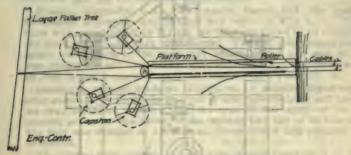
Fig. 18.—Arrangement of Capstans.
